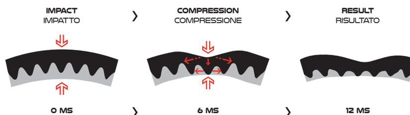
The innovative Conehead™ protection system comprises two layers of cone-shaped EPS of different densities. This allows the force generated by the impact to be dissipated over the entire surface of the helmet, significantly reducing head injuries.
